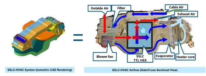
This project introduces a new system—SSLC (Sensible and Latent heat Separation Climate control system)—into the HVAC (Heating, Ventilation and Air Conditioning) unit that manages airflow within vehicles.
